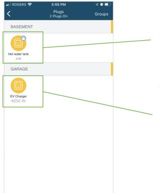
When a plug is "on" and shows as orange, it does not mean the device connected to the Plug is actually in use.
